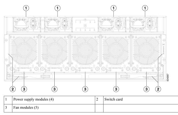
The following figure shows the port-side chassis features that you use when installing the chassis or replacing its modules.
