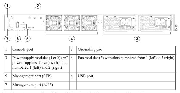
The fan and power supply modules are field replaceable. You can replace one fan module or one power supply module during operations so long as the other modules are installed and operating. If you have only one power supply installed, you can install the replacement power supply in the open slot before removing the original power supply.
