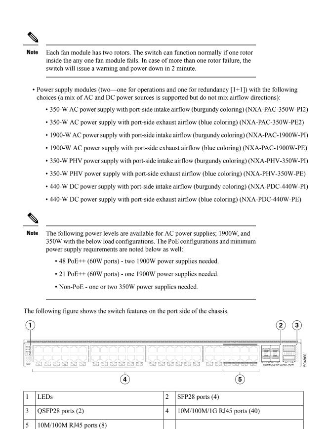
To determine which transceivers, adapters, and cables are support this switch, see the Cisco Transceiver Modules Compatibility Information document.
