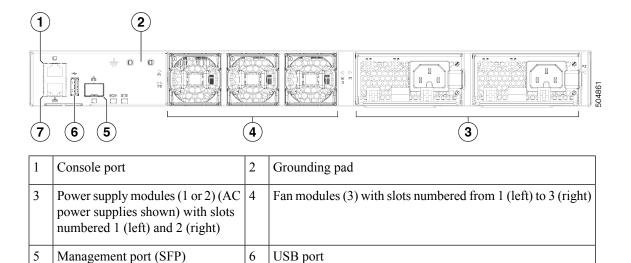
The figure shows the Cisco Nexus 9348GC-FX3 switch.
