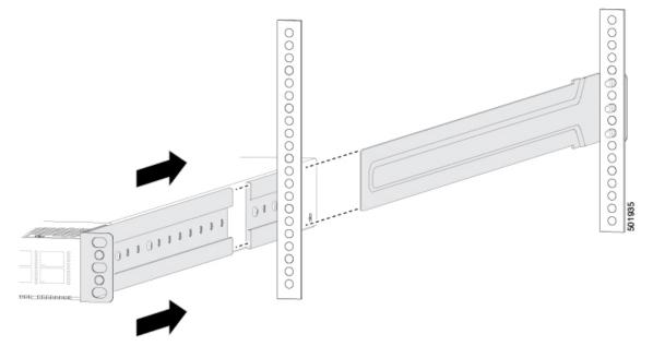
b) Align the two rear rack-mount guides on either side of the switch with the slider rails installed in the rack. Slide the rack-mount guides onto the slider rails, and then gently slide the switch all the way into the rack until the front rack-mount brackets come in contact with two rack or cabinet posts.
