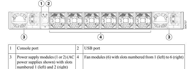
The following figure shows the side of the chassis.
