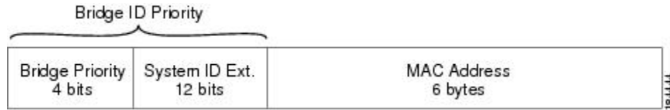
Figure 1: Bridge ID with Extended System ID
