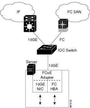
Cisco Nexus devices provide quality of service (QoS) capabilities to ensure lossless or best-effort service across the switch. For Fibre Channel traffic (FCoE) you should apply the lossless QoS classes. By default, best-effort service is applied to all of the Ethernet traffic. You can configure different QoS levels for specific classes of Ethernet traffic.
