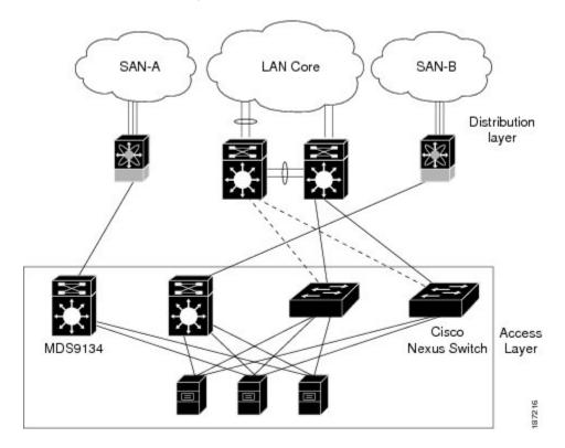
All of the server-side ports on the Cisco Nexus device are running standard Ethernet. FCoE is not required, so the server ports are connected using 10-Gigabit Ethernet NICs.
