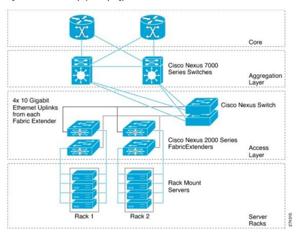
Figure 3: Fabric Extender Deployment Topology
