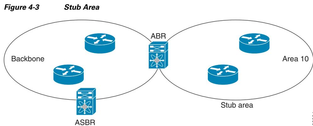
Stub areas use a default route for all traffic that needs to go through the backbone area to the external autonomous system. The default route is 0.0.0.0 for IPv4.
