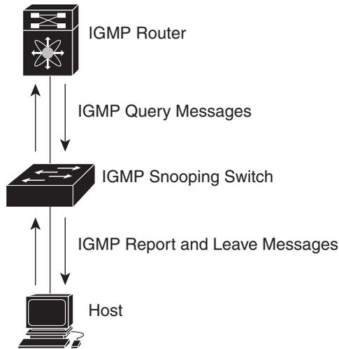
The IGMP snooping software operates upon IGMPv1, IGMPv2, and IGMPv3 control plane packets where Layer 3 control plane packets are intercepted and influence the Layer 2 forwarding behavior.
