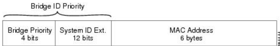
Figure 1: Bridge ID with Extended System ID
