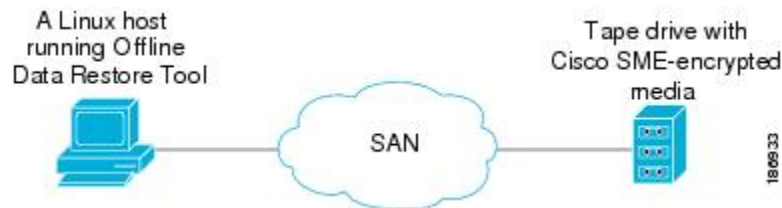
Figure 1: Offline Data Restore Tool (ODRT) Topology
