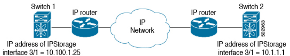
Figure 2-7 Assigning Profiles to Each IPStorage Interface
