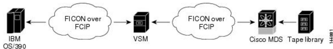
Figure 6: Host Accessing Standalone IBM-VTS (Virtual Tape Server) /STK-VSM (Virtual Shared Memory)
