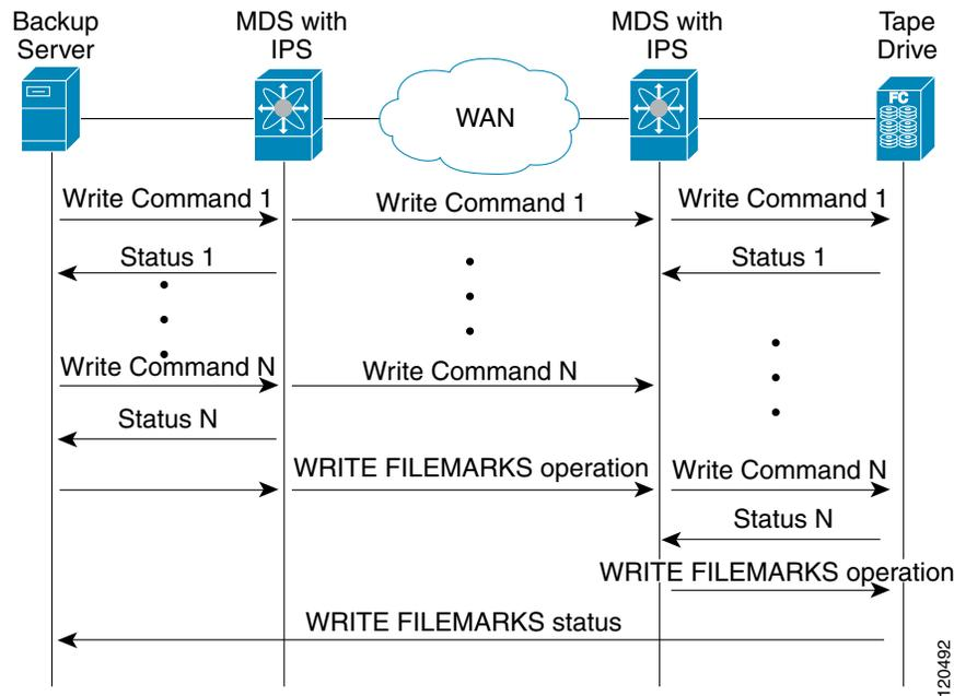
At the tape end of the FCIP or Fibre Channel tunnel, another Cisco MDS switch buffers the command and data it has received. It then acts as a backup server to the tape drive by listening to a transfer ready from the tape drive before forwarding the data.
