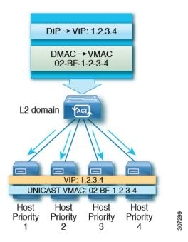
The use of a common MAC address would normally create a conflict, since Layer 2 switches expect to see unique source MAC addresses on all switch ports. To avoid this problem, Network Load Balancing uniquely modifies the source MAC address for outgoing packets. If the cluster MAC address is 02-BF-1-2-3-4, then each host's source MAC address is set to 02-*x*-1-2-3-4, where *x* is the host's priority within the cluster, as shown in the following figure.
