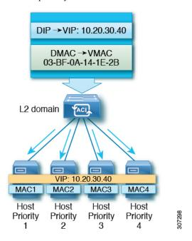
adapter's MAC address. For example, the multicast MAC address could be set to 03-BF-0A-14-1E-28 for a cluster's primary IP address of 10.20.30.40. Cluster communication doesn't require a separate adapter.
