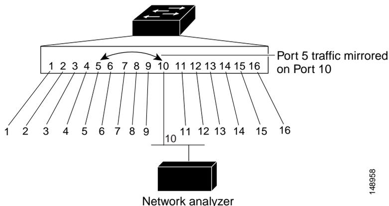
[Figure 29-2](#) is an example of a local SPAN in a switch stack, where the source and destination ports reside on different stack members.
