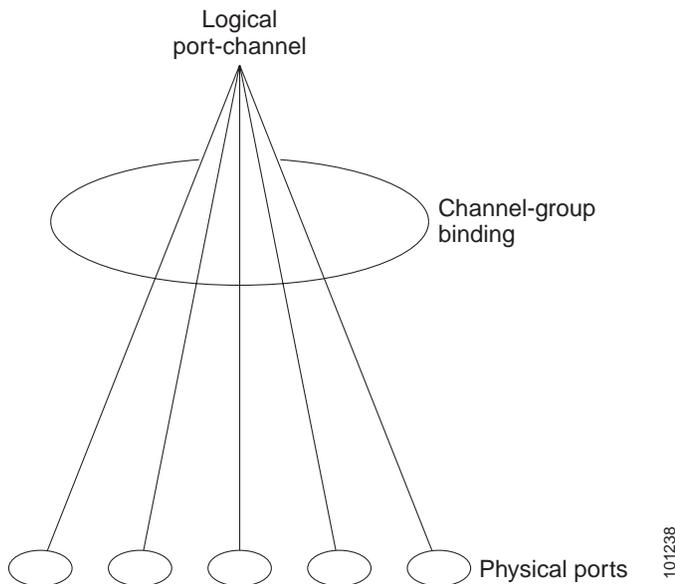
After you configure an EtherChannel, configuration changes applied to the port-channel interface apply to all the physical ports assigned to the port-channel interface. Configuration changes applied to the physical port affect only the port where you apply the configuration. To change the parameters of all ports in an EtherChannel, apply configuration commands to the port-channel interface, for example, spanning-tree commands or commands to configure a Layer 2 EtherChannel as a trunk.
