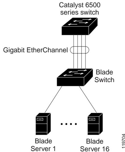
The EtherChannel provides full-duplex bandwidth up to 8 Gb/s (Gigabit EtherChannel) or 80 Gb/s (10-Gigabit EtherChannel) between your switch and another switch or host.
