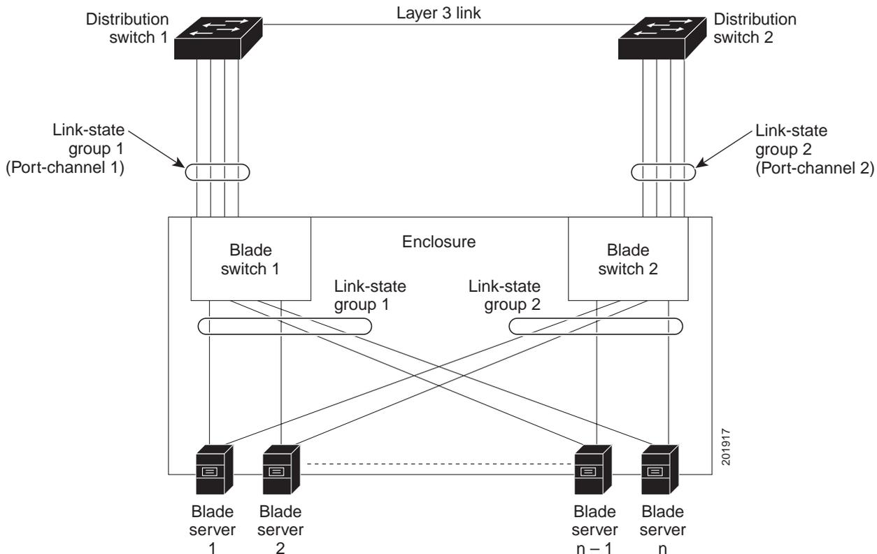
The configuration in [Figure 37-6](#) ensures that when server NIC adapter teaming is used, the traffic flow continues uninterrupted when the uplink connection to a distribution switch is lost.
