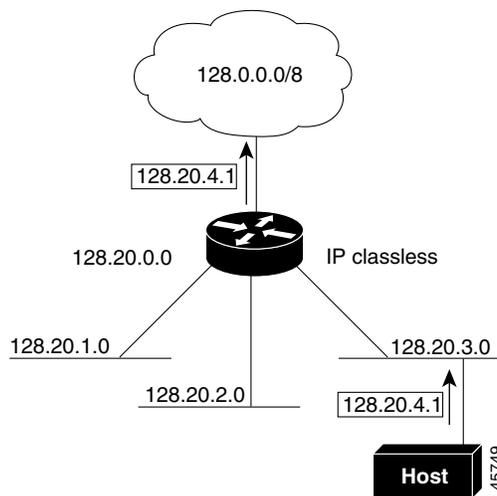
In [Figure 35-3](#), the router in network 128.20.0.0 is connected to subnets 128.20.1.0, 128.20.2.0, and 128.20.3.0. If the host sends a packet to 120.20.4.1, because there is no network default route, the router discards the packet.
