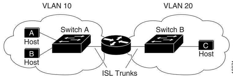
When Host A in VLAN 10 needs to communicate with Host B in VLAN 10, it sends a packet addressed to that host. Switch A forwards the packet directly to Host B, without sending it to the router.
