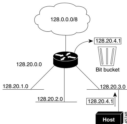
To prevent the switch from forwarding packets destined for unrecognized subnets to the best supernet route possible, you can disable classless routing behavior.
