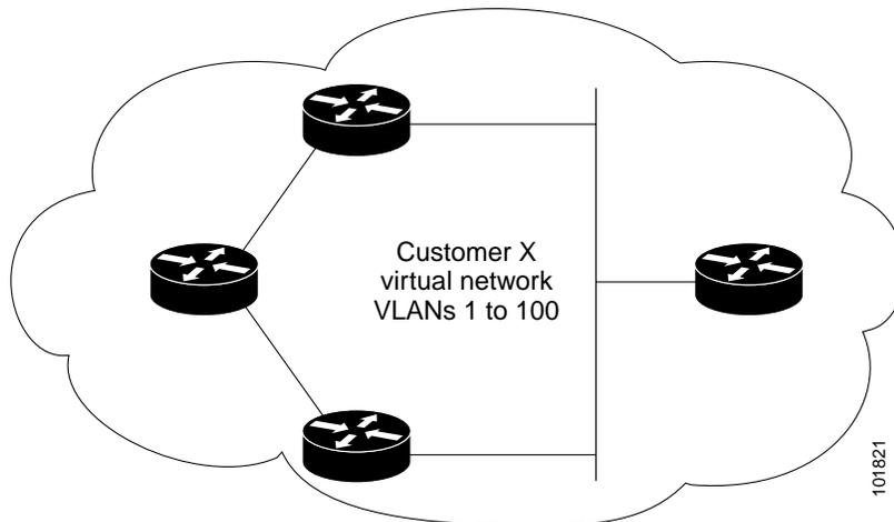
In an SP network, you can use Layer 2 protocol tunneling to enhance the creation of EtherChannels by emulating a point-to-point network topology. When you enable protocol tunneling (PAgP or LACP) on the SP switch, remote customer switches receive the PDUs and can negotiate the automatic creation of EtherChannels.
