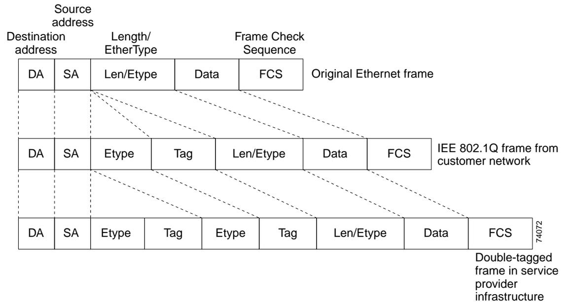
When the packet enters the trunk port of the service-provider egress switch, the outer tag is again stripped as the switch internally processes the packet. However, the metro tag is not added when the packet is sent out the tunnel port on the edge switch into the customer network. The packet is sent as a normal IEEE 802.1Q-tagged frame to preserve the original VLAN numbers in the customer network.
