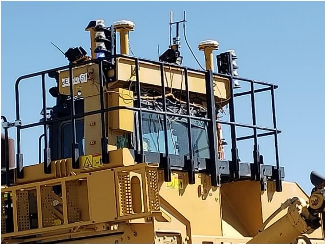
Figure 12. Dozer Top-Mount Radio Installation
