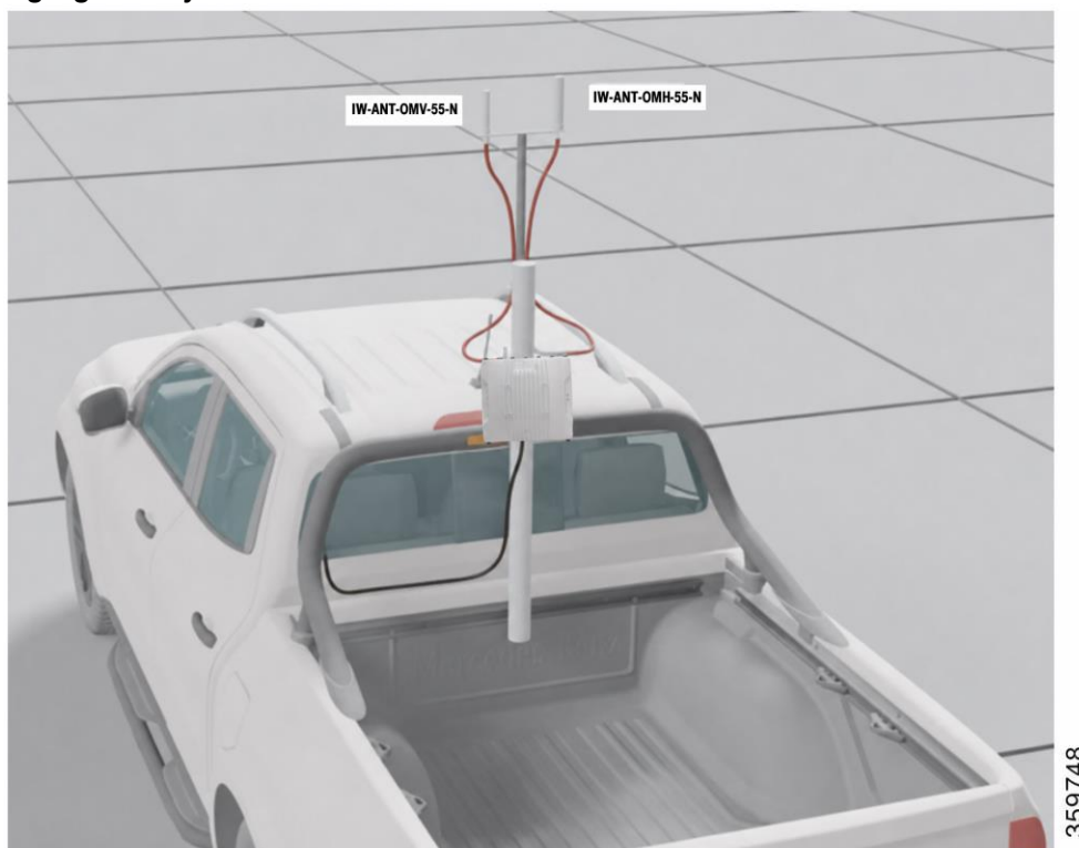
Figure 10. Mining Light Utility Vehicle Radio Installation
