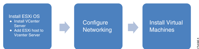
Figure 6 Flow Diagram for Virtualization Configuration
