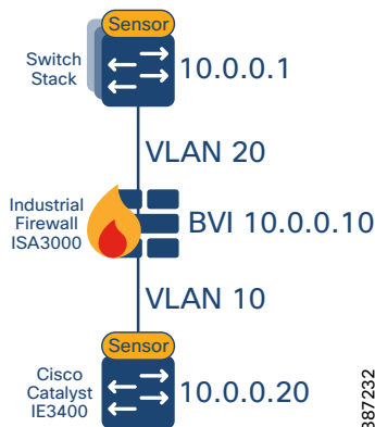
Figure 21 Transparent Mode with BVI Interface
