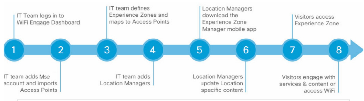
Figure 1-1 Process Flow for the WiFi Engage
