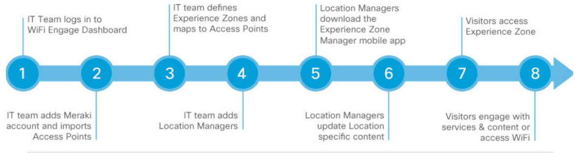
Figure 1-1 Process Flow for the WiFi Engage
