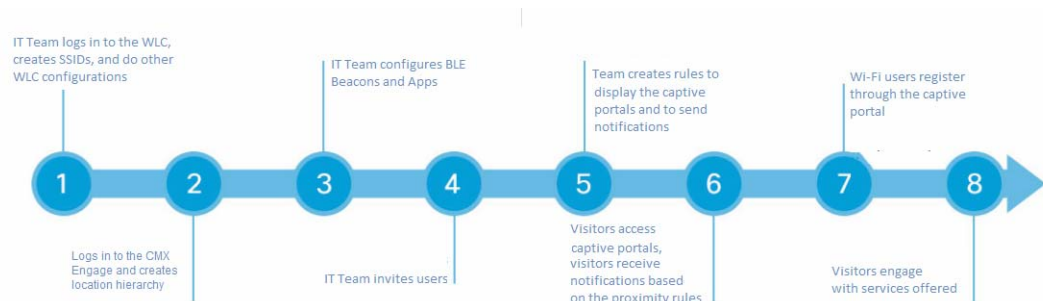
Figure 1-2 Process Flow for the CMX Engage
