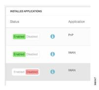
Step 5 Click Enabled for the new IWAN application. APIC-EM enables the new version. When upgrading from a previous version of the IWAN app, APIC-EM preserves the existing IWAN configuration.
