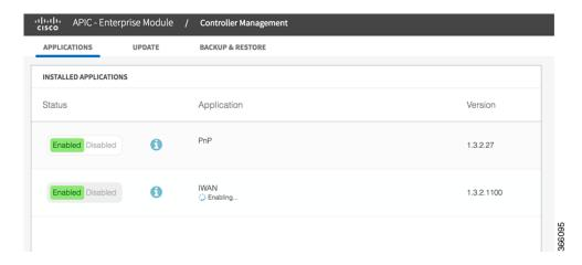
Step 6 When the installation and enabling are complete, clear the browser cache and refresh the APIC-EM Applications page. The Status column shows that the new IWAN app is enabled, and the Version column shows the new IWAN app version. Any previous version of the IWAN app is removed from the list. (The example below shows an earlier release of the IWAN app.)
