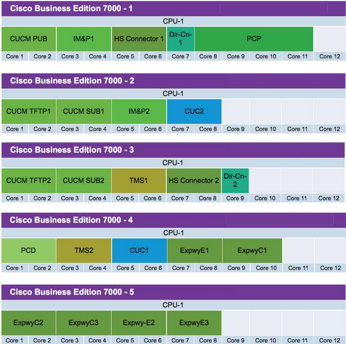
Figure 7-3 Virtual Machine Placement Example using VMPT
