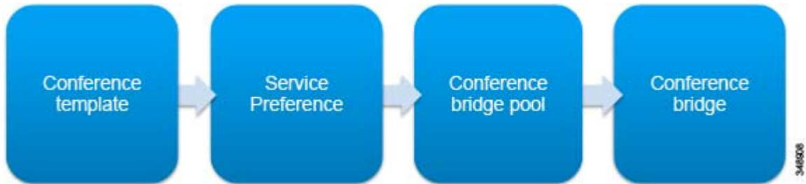
Figure 3-9 TelePresence Conductor Internal Configuration Flow for Instant Conferences
