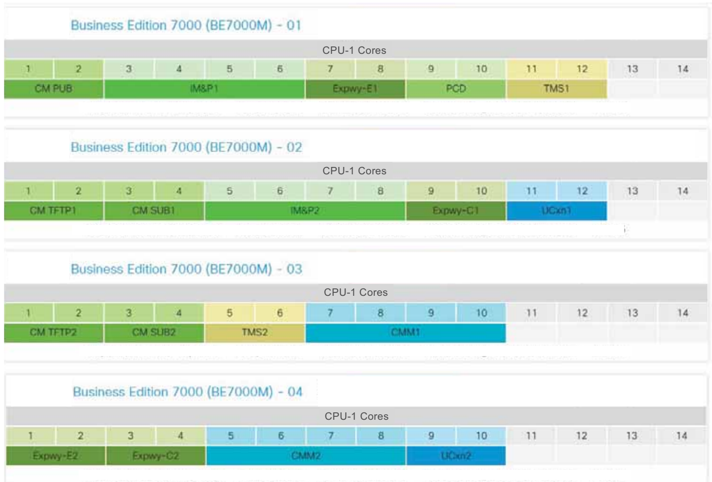
Figure 9-1 Virtual Machine Placement Example Using Quote Collab
