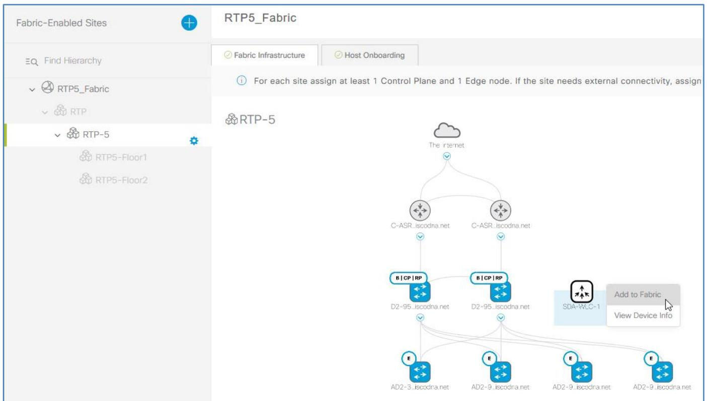
**Step 2.** At the bottom of the screen click **Save**, in the slide-out menu keep the default selection **Now**, and then click **Apply**. The WLC configurations are created to establish a secure connection to the fabric control plane nodes.
