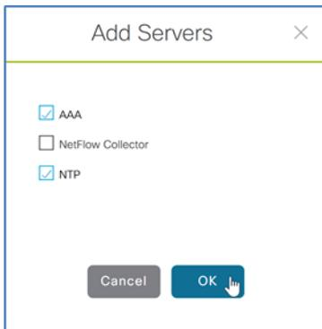
The configuration pane is updated with **AAA Server** and **NTP Server** as available configuration sections. You configure AAA services for both the network infrastructure device administration and the client endpoints connecting to the infrastructure. For this example, the high-availability standalone ISE nodes are used.
