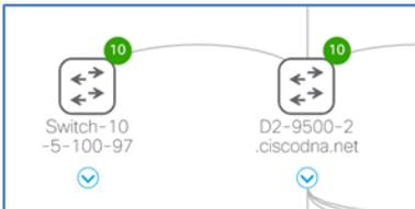
**Step 8.** Navigate to **PROVISION > Devices > Inventory**. At the top, click the **LAN Automation** drop-down, click **LAN Auto Status**. After the devices discovered all reach **Completed** state, click **Stop**. LAN Automation tears down all Layer 2 connectivity on VLAN 1 and the underlay IS-IS routing process is used for reachability to the discovered devices, and these devices are added and managed in Inventory.
