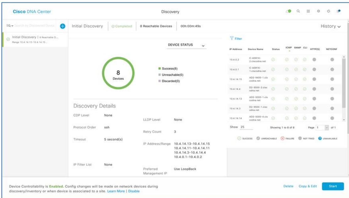
**Step 4.** If there are any discovery failures, inspect the devices list, resolve the problem, and restart the discovery for those devices along with any additional devices to add to the inventory.
