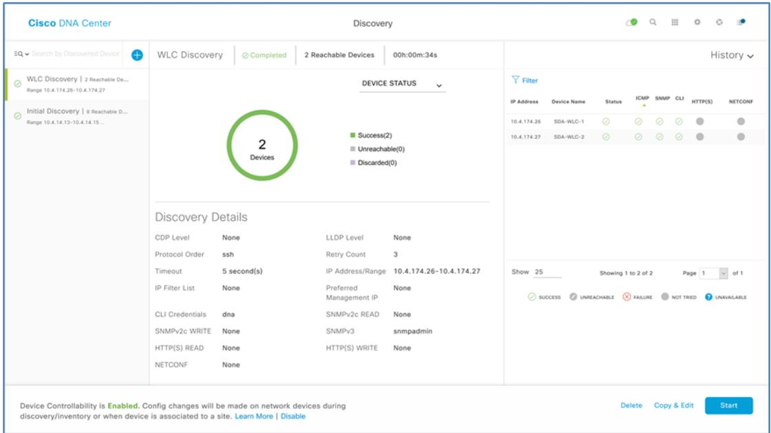
**Step 4.** If there are any discovery failures, inspect the devices list, resolve the problem, and restart the discovery for those devices along with any additional devices to add to the inventory.
