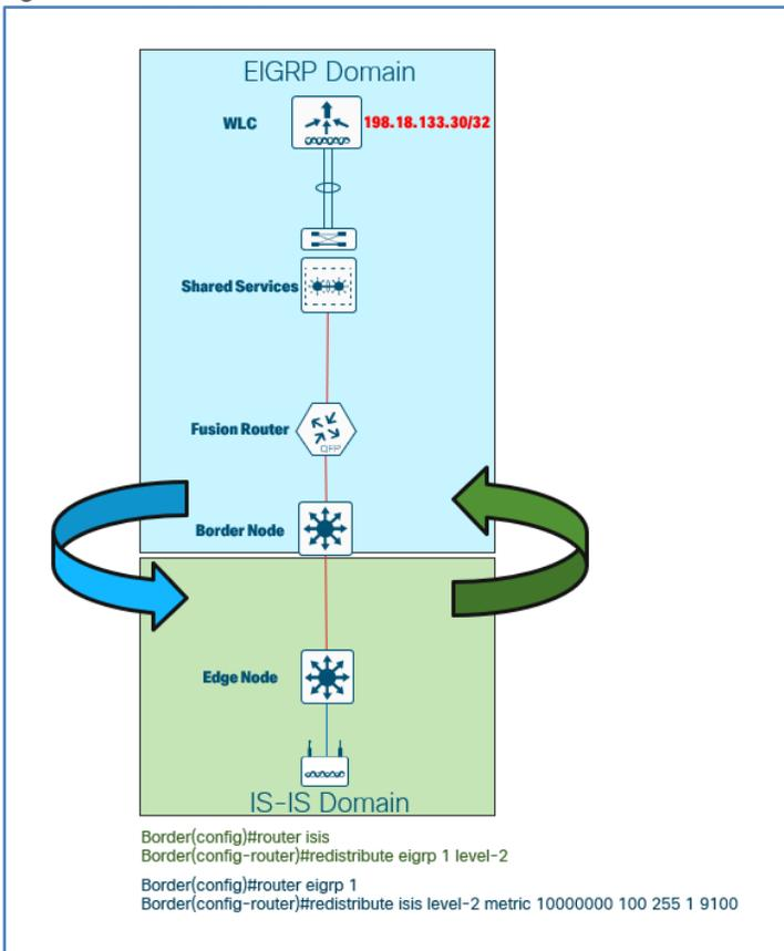
From the perspective of the border node, the WLC is reachable via EIGRP with an administrative distance of 90. From the perspective of the edge node, the WLC route is redistributed into IS-IS which as a default administrative distance of 115.
