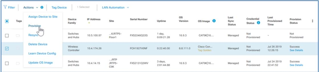
**Step 2.** Assign the site (example: Global/RTP/RTP-5), click **Next**, at the **Configuration** step under **Managed AP Location** select the additional floor assignments for APs managed by the WLC (example: Global/RTP/RTP5-C9K/Floor 1), click **Next**, and then at the **Advanced Configuration** step click **Next**.
