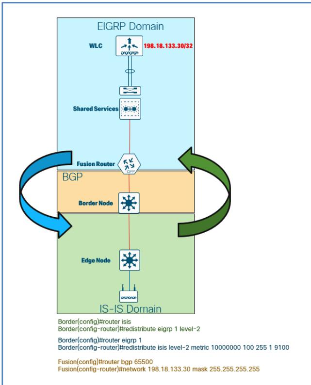
The result is that the WLC's subnet is known through both BGP and through EIGRP. BGP has an administrative distance of twenty (20) which will result in its route in routing table instead of the route from EIGRP.
