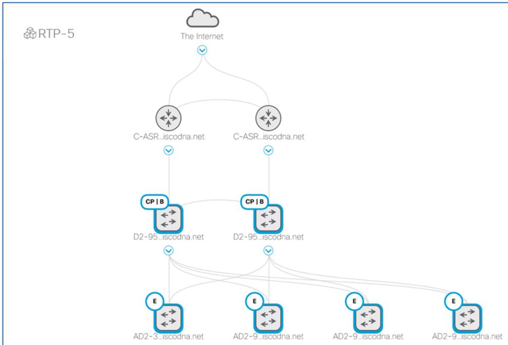
The fabric icons turn blue, signaling your intent to create the fabric. Actual provisioning of the devices can take longer to complete.
