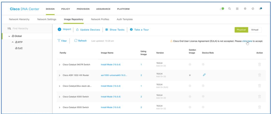
**Step 2.** Under the **Image Name** column click the down arrow next to the image listed for a device family, and then click the **Golden Image** star to mark the appropriate image as the preferred one for the platform.
