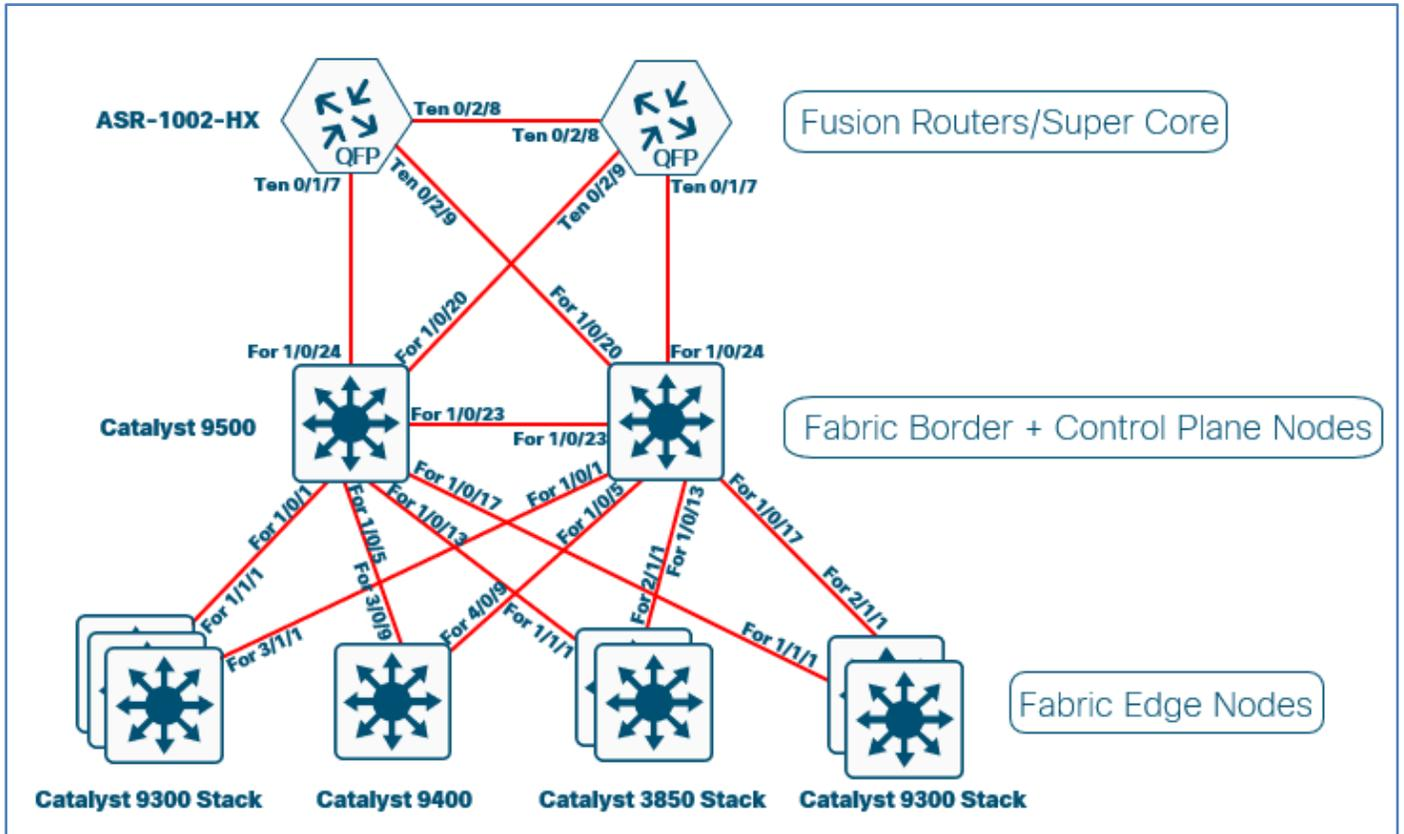
**Step 1.** Configure the switch connections within the underlay network infrastructure. Repeat this step for every link to a neighbor switch within the fabric underlay. If the underlay device will be provisioned as a fabric border node and the connection is to be used as a handoff from the fabric to the external infrastructure, then use the next procedure instead.
