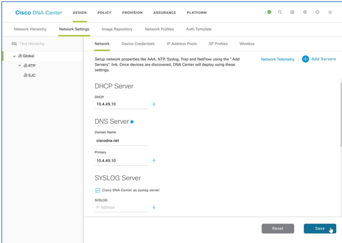
**Step 2.** Near the top, next to **Network Telemetry**, click the **+ Add Servers** button, select the **AAA** and **NTP** check boxes, and then click **OK**.
