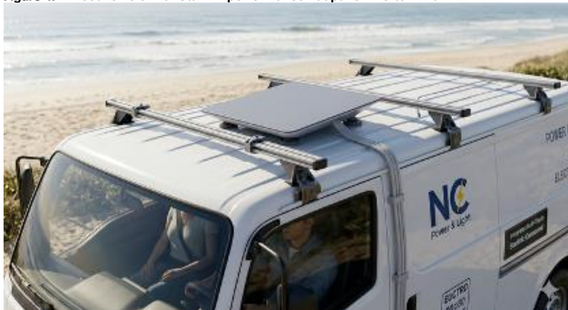
Figure 4. Fleet vehicle with Starlink performance flat panel LEO terminal
