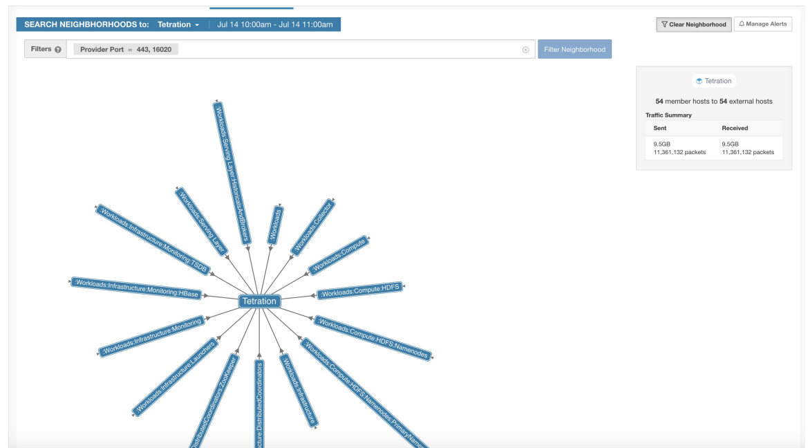
Figure 77: Example: Filter input supports “,” for Ports
