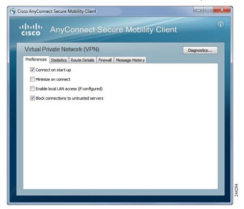
If the user un-checks **Block connections to untrusted servers**, and the only issue with the certificate is that the CA is untrusted, then the next time the user attempts to connect to this secure gateway, the user will not see the Certificate Blocked Error Dialog dialog; they only see the following dialog:
