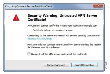
If the user checks **Always trust this VPN server and import the certificate**, then future connections to this secure gateway will not prompt the user to continue.
