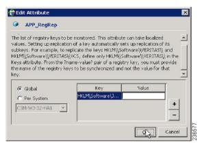
Note Security Manager stores client user preferences in the server registry under HKEY\_LOCAL\_MACHINE\SOFTWARE\JavaSoft\Prefs\vms. The registry replication agent (RegRep) monitors changes to the specified registry location on the active server and synchronizes these changes to a secondary server in the event of a failover.
