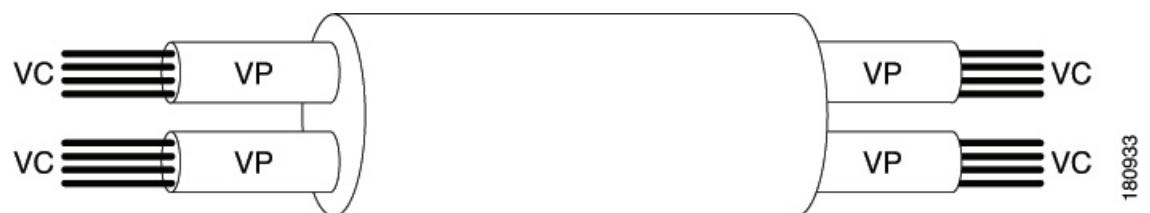
Figure 2: ATM Virtual Path and Virtual Channel Connections
