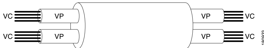
Figure 62-2 ATM Virtual Path and Virtual Channel Connections
