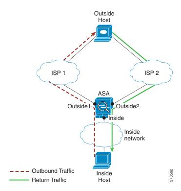
**Non-Zoned Problem**: The ASA maintains the connection tables on a per-interface basis. When the returning traffic arrives at Outside2, it will not match the connection table and will be dropped.
