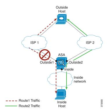
**Non-Zoned Problem**: The connection between the inside and outside host will be deleted; a new connection must be established using a new next-best route. For UDP, the new route will be used after a single packet drop, but for TCP, a new connection has to be reestablished.
