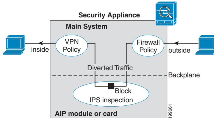
The next illustration depicts traffic flow when the IPS module is running in Promiscuous mode. In this example, the IPS module sends a shun message to the ASA for traffic it has identified as a threat.
