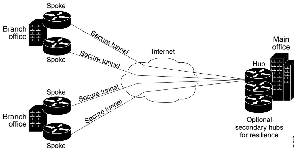
This topology usually represents an intranet VPN that connects an enterprise's main office with branch offices using persistent connections to a third-party network or the Internet. VPNs in a hub-and-spoke topology provide all employees with full access to the enterprise network, regardless of the size, number, or location of its remote operations.
