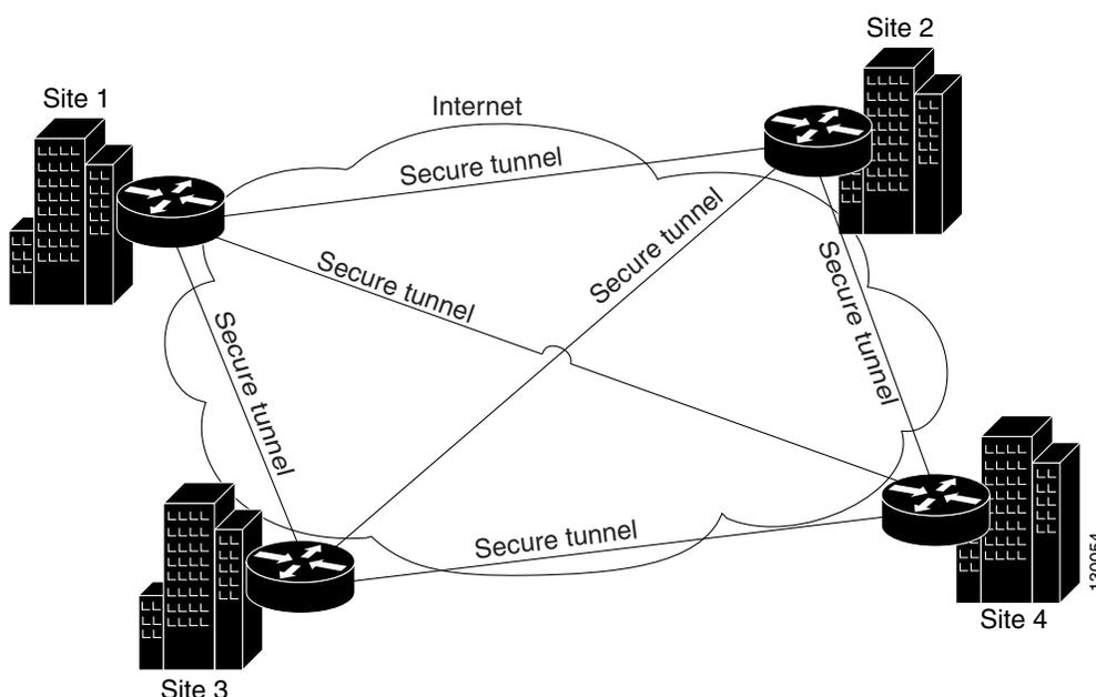
A full mesh network is reliable and offers redundancy. When the assigned technology is GRE and one device (or node) can no longer operate, all the rest can still communicate with one another, directly or through one or more intermediate nodes. With regular IPsec, if one device can no longer operate, a crypto access control list (ACL) that specifies the protected networks, is created per two peers.
