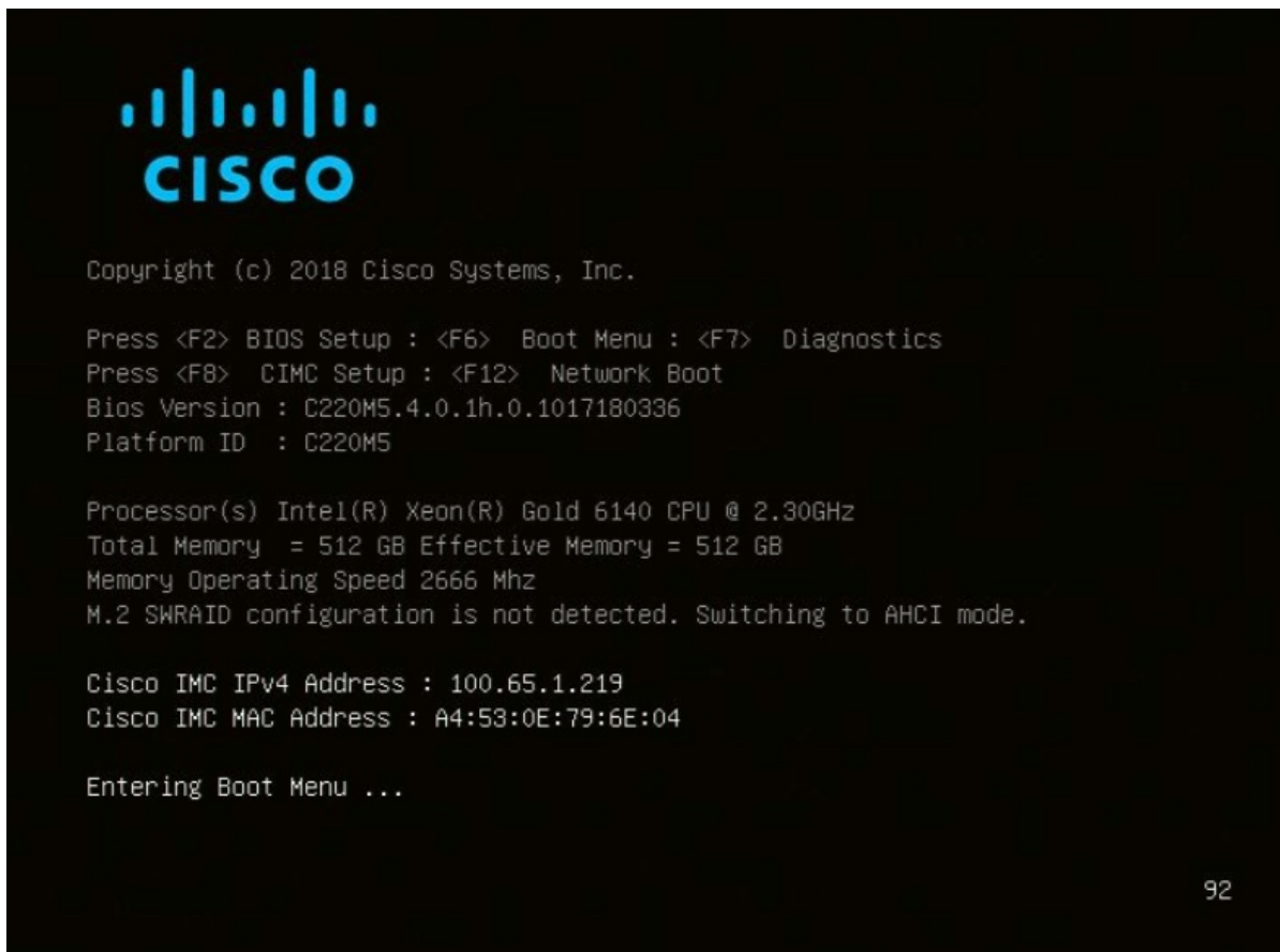
Figure 3: BIOS Window - Choose Boot Menu <F6> for Recovery Mode
