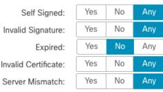
In the following example, traffic would match this rule condition if the incoming traffic is using a certificate that has an invalid issuer, is self-signed, expired, and it is an invalid certificate.
