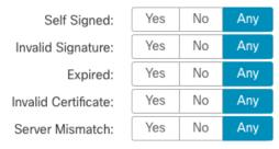
The following figure shows a certificate status rule condition checking for the absence of a status. In this case, because of the configuration, it matches against traffic encrypted with a certificate that has not expired and monitors that traffic.
