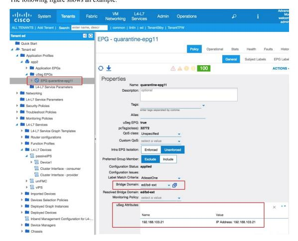
The figure shows that a device at IP address 192.168.100.21 has been quarantined.
