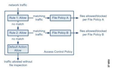
The policy has two access control rules, both of which use the Allow action and are associated with file policies. The policy's default action is also to allow traffic, but without file policy inspection. In this scenario, traffic is handled as follows:
