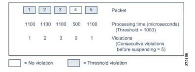
In the above example, the time required to process each of the first three packets violates the rule latency threshold of 1000 microseconds, and the violations counter increments with each violation. Processing of the fourth packet does not violate the threshold, and the violations counter resets to zero. The fifth packet violates the threshold and the violations counter restarts at one.
