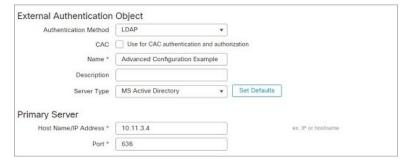
This example shows a connection using a base distinguished name of OU=security, DC=it, DC=example, DC=com for the security organization in the information technology domain of the Example company. However, note that this server has a base filter of (cn=\*smith). The filter restricts the users retrieved from the server to those with a common name ending in smith.
