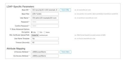
The connection to the server is encrypted using SSL and a certificate named certificate.pem is used for the connection. In addition, connections to the server time out after 60 seconds because of the **Timeout (Seconds)** setting.
