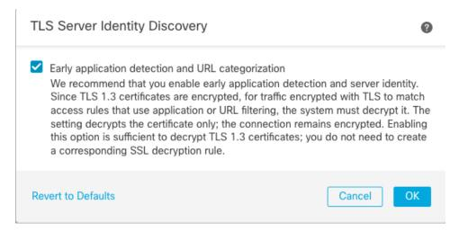
We strongly recommend enabling it for any traffic you want to match on application or URL criteria, especially if you want to perform deep inspection of that traffic. An SSL policy is not required because *traffic is not decrypted* in the process of extracting the server certificate.
