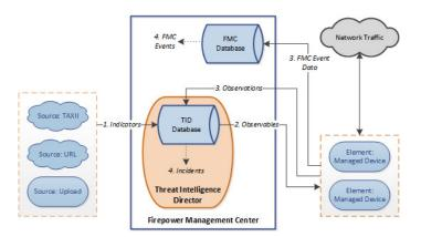
When a TID incident is fully or partially realized, the system takes the configured *action* (monitor, block, partially block, or no action). For details, see Factors That Affect the Action Taken, on page 22.
