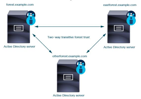
Finally, you can set up the FMC to be able to enforce identity policies on users and groups in a two-forest system with two-way transitive forest trust. Suppose each forest has at least one domain controller, each of which authenticates different users and groups. For the FMC to be able to enforce identity policies on those users and groups, you must set up each domain containing relevant users as FMC realm and each domain controller as FMC directory in the respective realm.
