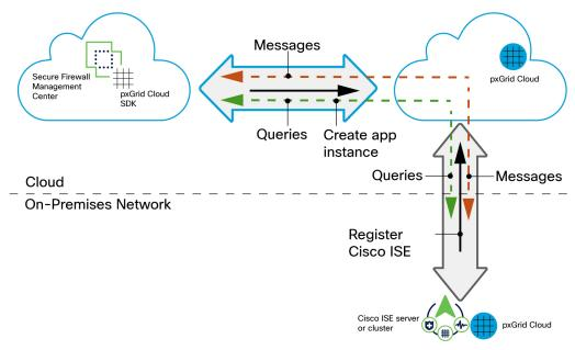
Your Secure Firewall Management Center uses the pxGrid Cloud SDK to programmatically retrieve user information from an on-premises Cisco ISE server or cluster so these users can be used in identity policies on the Secure Firewall Management Center.
